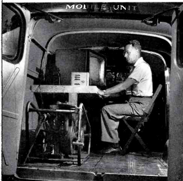
WEEU-TV, Reading, Pa. Harold E. Scheerer, Asst. Dir. of Tech. Operations, uses equipment in the station's mobile unit to measure the field strength of the broadcast signal from any given point within the wide radius of the station's transmitter.
